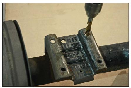
49. Position lower axle brackets onto rearend-housing spring plates. Place the 1/2" U-bolts over the axle tube and through the holes in the axle bracket. Secure with flat washers and locknuts. Tighten evenly to 60 lb-ft.
