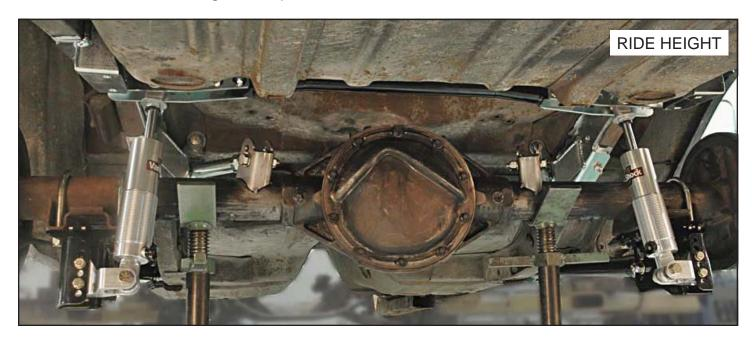
70. Using a jack, cycle the rear suspension through its full range of vertical travel and body roll in both directions to check for binding and potential clearance issues at all suspension joints and along the lengths of any moving parts including the rearend housing. Remember the ShockWave® will be larger in diameter when inflated. Allow for an additional 1/2" to 3/4" of clearance around the air spring.
