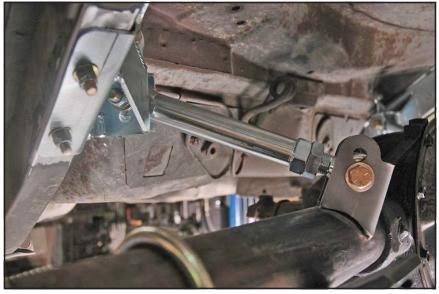
57. Install the billet lower-shock mounts at the lower axle bracket using 3/8" hardware. Leave one blank hole below the mount for initial setup.
