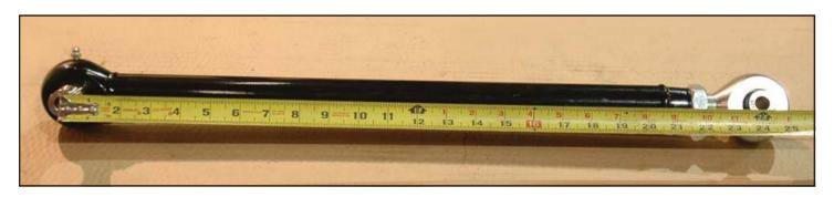
51. Install the lower suspension links at the factory front leaf spring mount using 1/2" diameter bolts, flat washers, and locknuts.
