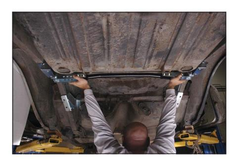
27. Use a die grinder, grinding-cone drill attachment, or file to enlarge the oval holes up to the scribe marks on the frame rails.
