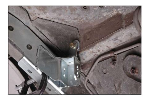
35. Verify the shock bracket channel edge is the same distance from the flat vertical section of the undercarriage. Ours measured 10-1/2".
