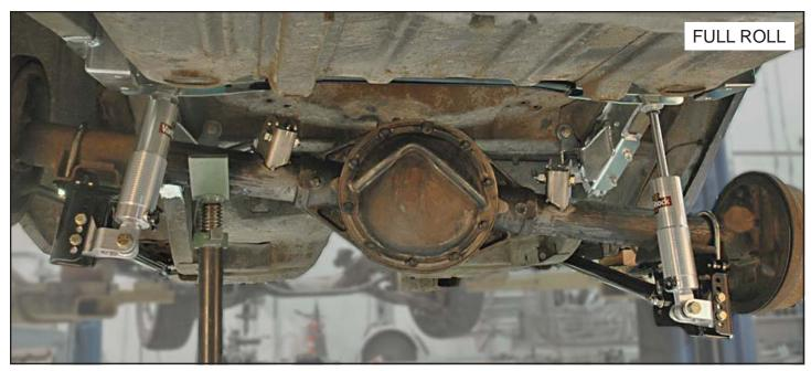
71. Once clearance has been verified, remove the housing and final weld the upper link brackets to the housing.
