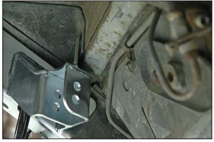
18. Place the flat washer over the 3/8-24 x 1-3/4" hex bolt and insert through the forward mount tabs, shims, and through the floor behind the seat.
