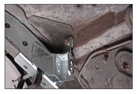
21. Verify the cradle frame brackets are clamped tightly against the inside and bottom surfaces of the frame rails.
