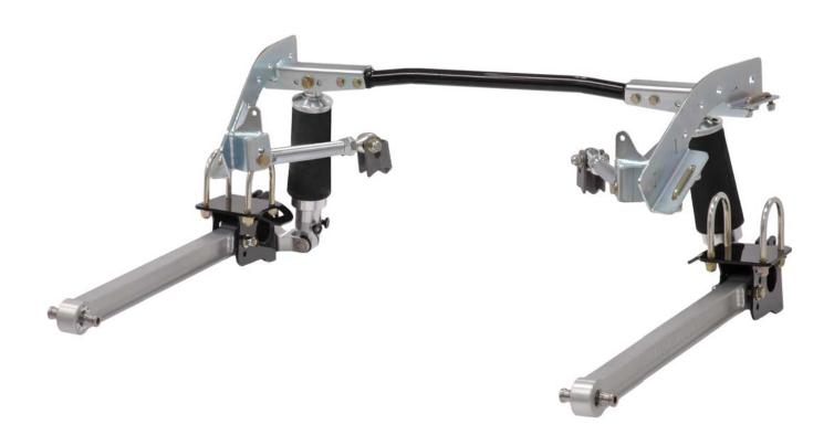
**Description:** Canted 4-bar rear air suspension for 1967-1969 Camaro and Firebird. Includes upper links, lower links, suspension cradle, axle brackets, and VariShock ShockWaves.
