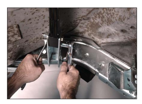
23. Clearly mark the weld-prep areas onto the undercarriage by scribing guidelines onto the surface of the frame rail. Scribe the overall outline of the bracket, the holes along the inside of the frame rail, and finally the eight oval holes along the bottom of the frame rail.
