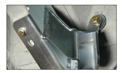
21. Verify the cradle frame brackets are clamped tightly against the inside and bottom surfaces of the frame rails.
