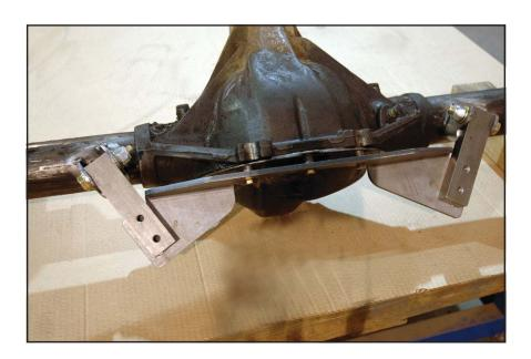
49. Use a 1/2" diameter drill bit to enlarge the holes in the factory spring plates for the u-bolts.
