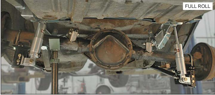
72. Once clearance has been verified, remove the housing and final weld the upper link brackets to the housing.
