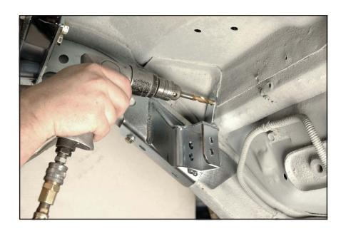
17. Check for a gap between the forward mount tabs and body panel. If there is a gap, use the supplied fender washers as shims to fill the gap and create a stable fit for the cradle.
