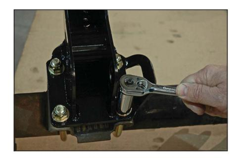
51. Adjust the lower link bars to 24" center to center of the mounting holes, if applicable.
