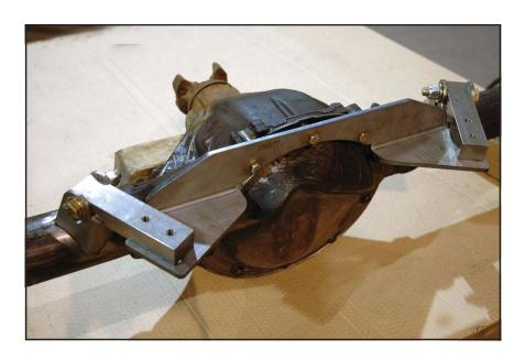
48. When leaving the rearend cover on the housings use the provided spacers. Also make sure the bracket bosses are at the forward holes. If welding with the cover removed the spacers are NOT used and the bracket bosses are mounted in the rear holes. Only tack weld the brackets at this time.
