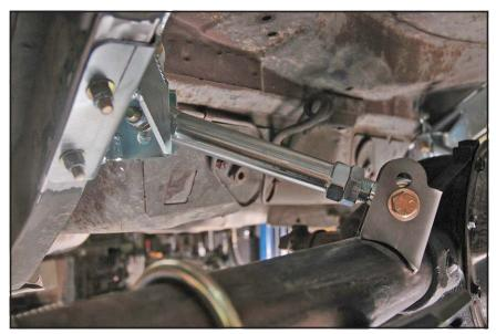
58. Install the billet lower-shock mounts at the lower axle bracket using 3/8" hardware. Leave two blank holes below the mount for initial setup.
