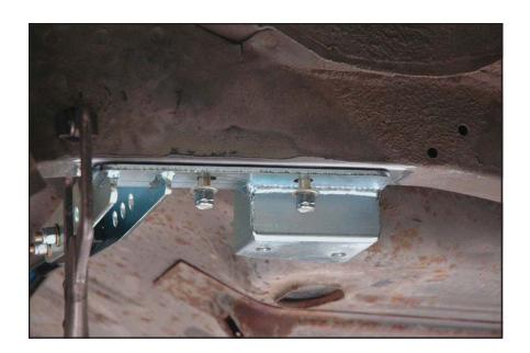
38. Using the same procedure, install the u-bolt in the frame brackets closest to the front of car.
