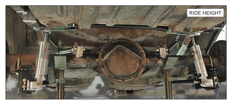
71. Using a jack, cycle the rear suspension through its full range of vertical travel and body roll in both directions to check for binding and potential clearance issues at all suspension joints and along the lengths of any moving parts including the rearend housing. Remember the ShockWave® will be larger in diameter when inflated. Allow for an additional 1/2" to 3/4" of clearance around the air spring.
