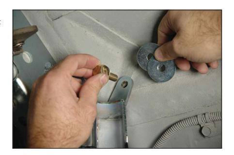
19. Secure the bolt from inside the vehicle with a 3/8" flat washer and locknut. The rear seat must be removed for this step. In some cars the flange behind the seat my need to be bent to allow the hardware to be tightened.
