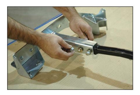
Use C-clamps on the frame brackets to hold them firmly in place.
