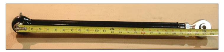
52. Install the lower suspension links at the factory front leaf spring mount using 1/2" diameter bolts, flat washers, and locknuts.
