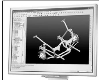
**Product systems, such as this bolt-on Chevy II drag race strut clip, are built as assembled computer models, which can then be used to develop manufacturing fixtures and test various product options.**
