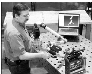
**The FaroArm laser scanner is just one of the computerized measurement devices in Chassisworks' high-tech tool bin. With point and shoot ease, Chassisworks' laser scanner picks up fine details, such as casting imperfections, threads, and even tooling marks.**
