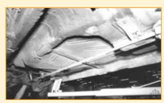
Reference points are also critical under the car for fabricating the new subframe; in this instance, the front of the transmission crossmember-mount is the fixed point choice used for measuring back to the front of the axle housing.
