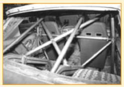
tab for the window net was welded right next to the gusset at the intersection of the main hoop and the cage side; the lower, rear tab was mounted to the main hoop, as shown. Here, the proper location for the clevis for the quick-release pin is determined.
