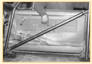
After cutting the side bar to length and installing the upper clevis, but before everything was welded up, the door was closed to make sure that the side bar didn't interfere with the operation of the door and window handles. As shown here, the handles are fine; however, the stock arm rests are history.
