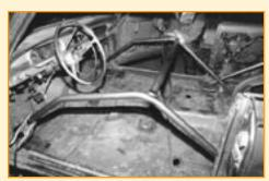
Here's the aforementioned method for welding the top of the windshield-brace joint. The tack welds holding the cage-side/ windshield-brace assembly to the floor and to the main hoop are broken, the assembly is set down on the floor, and the welding can be easily done. (The tacks holding the main hoop to the floor will probably also have to come loose for this process.)
