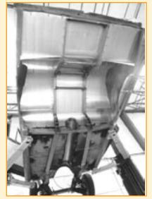
With the Nova high on the lift of our in-house chassis shop, this snail's-eye view shows how the tin installation, the dropped crossmember, and the subframe connectors all tie in together to provide a sanitary package.
