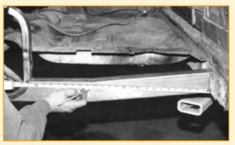
The front crossmember is then also marked for the frame-rail locations. The 24-inch frame width is subtracted from the length of the dropped crossmember, that number is divided by two, and this distance is measured in from the rocker panel on each side.
