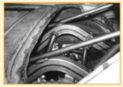
After welding the struts front and back, they were also welded to the raised part of the subframe rails since they line up so closely in this early Nova kit.
