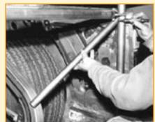
The next order of business is to fabricate the struts from the main hoop back to the new subframe rails. With the lower end of the tubing roughly in place on the top of the subframe bend, the top of the tube is marked with the angle required to have it fit fairly snugly under the back-brace mount.
