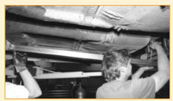
After the frame stub is removed, the 3x2-inch box tube to be used for the connector is held up in place and the trailing end marked for cutting. As always, a snug fit aids in the installation process.
