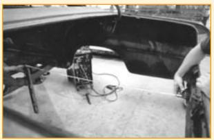
Next, the distance from the trailing edge of the crossmember to the inside of the rear of the car, in the trunk area, is determined. The rails will rest on the lip left behind when the trunk was cut out.
