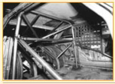
This view into the Nova's passenger compartment shows all the tubing of the 10-point roll-cage kit in place at the completion of the project.
