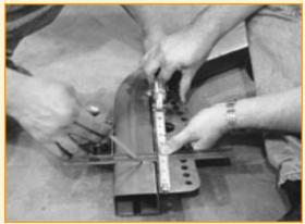
The first step in preparing the new frame rails for installation is to cut the vertical section of the front of the rails to size. The 4-link brackets are designed to fit flush with the bottom of the front crossmember; the frame rail will be cut three inches up from the bottom of the 4-link bracket, which is designed to fit up snug in the frame rail's curve.
