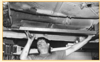
The floor of the Nova needed only a few taps with a mallet to make room for the connectors, while some other cars will require the floor to be notched. Note that the connector fits under the "overhang" of the frame rail, and is lined up with its inside edge.
