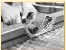
The cut in the crossmember was cleaned up with a sanding drum, which helped achieve a perfect fit for the driveshaft loop.
