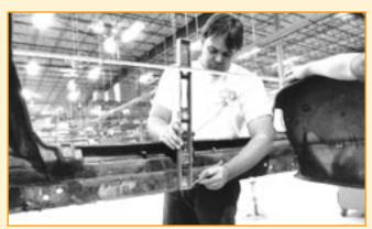
Assuming the body is unwrinkled and the rear quarter panels are straight, a tape is used to measure across the back of the car to find the exact center of the rear area. It can't be assumed that the trunklatch mechanism is in the middle of the car.
