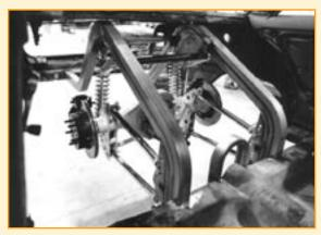
This is an overall view of the completed 4-link rear subframe and suspension system from the passenger compartment...
