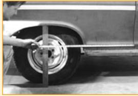
The first step in a project to upgrade the rear suspension of any car is to make sure that the axle centerline will end up back where it started. Here, a measurement is taken (and recorded) of the stock location, using the door opening as the point of reference.
