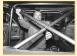
The next chore is the fabrication of the X-braces. The area at the top of the antiroll-bar mount was designated as the spot to mount the rear of the brace, while the forward end will attach right in the middle of the main-hoop bend, in line with the cage-side tubing. After the first, continuous-length brace was cut, formed and tacked to the car, the second piece of X-brace tubing is marked to start its fitting procedure.
