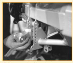
The billet, CNC-machined lower shock mounts are installed on the housing, again starting off by using the middle set of bracket holes.
