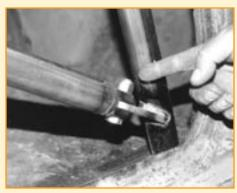
The nut has to be located at the top in this case, or the bar will never be able to be removed. The angle and position of the lower mount must also allow the intended operation of the swing-out arm.
