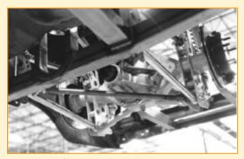
...while this shot from under the car shows the track locater in place, along with how the subframe connectors meet the crossmember.
