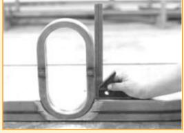
After the loop is cut to size and the two halves welded together, it is tacked to the crossmember. Again, the use of a square helps in final positioning.
