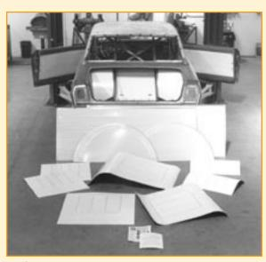
All of the pieces used in a typical tin-installation project are laid out here, including the detailed instruction sheets.
