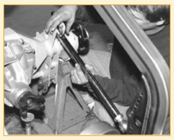
With the housing resting roughly in place and the pinion angle established with the help of a protractor and screw-type jackstand, it's time to install the link bars. The middle set of holes on each bracket is used for the initial set up, and all the bars are positioned with their threaded rod ends in the forward location, to facilitate later fine-tuning of the suspension.
