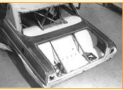
The installation of interior tin is covered elsewhere in this catalog, but this is what the interior of the Nova looked like when it was fully skinned. All panels are aluminum, and still covered with the protective plastic; the driveshaft tunnel is steel and welded to the floor. Cleco clips are being used to hold the panels in place, prior to the actual riveting.
