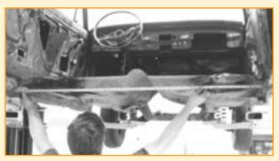
The crossmember will reside between the rocker panels of the unibody Nova, along the lower edge. When measuring for the proper width of the crossmember, be sure to note the location of the driveshaft centerline, which is rarely in the exact center of the car.
