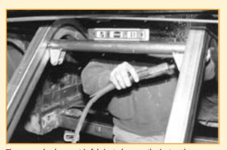
The upper shock mount is fabricated as per the instructions, positioned as referenced from the dropped crossmember, and tacked to the frame rails. (The use of a level that attaches to the tubing magnetically is recommended, but you must make sure that there are no metal shavings between the level and the tubing.)
