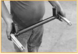
Our exclusive antiroll bar was also installed in the Nova. This is the completed assembly after it was fabricated; the box-tube mounting brackets fit inside of, and are welded to, the new subframe rails, while the width of the arms exactly matches the outer width of the frame. Pieces of thin steel plate are included for capping off the cut-to-size mounting brackets.
