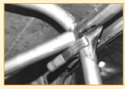
These clamps also come in very handy to keep the various pieces of tubing in place during the fitting process. Also visible is one of the gussets that are installed at the intersection of each cage side and the main hoop.
