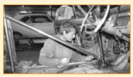
Because this Nova will be seeing considerable street time, swing-out side bars are being installed along with the removable back brace. Here, the swing-out clevis is welded to the lower end of the tube, bolted to the mounting tab, and, with the top end of the tube resting roughly in place, the tab is about to be tacked to the cage-side tubing.
