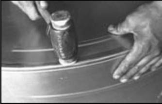
**17** With the rest of the protective plastic peeled away, a hammer is used to complete the bead.
