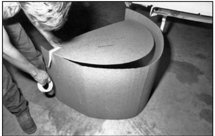
**7** Now the two cardboard sections are joined together with strips of masking tape.
