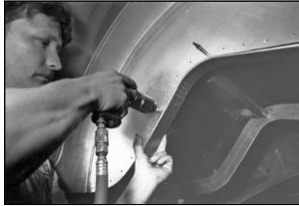
**18** Each fully trimmed tub can be temporarily clamped or clipped to the frame while mounting holes are drilled 1" up from the frame, 2" apart for mounting rivets. (Note the Cleco pin attaching this tub at the frame's bend.)
