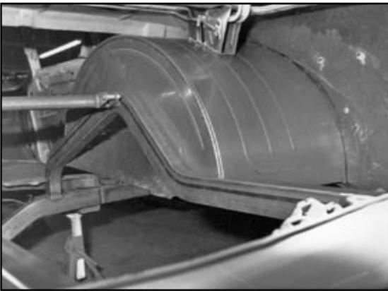
**21** Careful forward positioning of the new tub ensured uninterrupted operation of the original '57 Chevy trunk hinges. (In other applications, some modification of the stock hinges may be required.)
