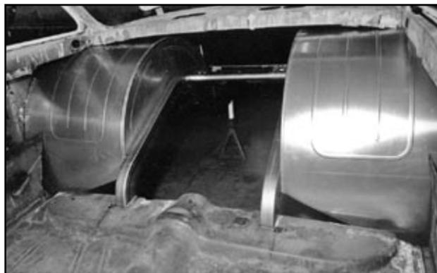
**22** Here's a hot rodder's version of a "hot tub in the back." Together with a universal Chassisworks subframe, the new tubs nearly doubled this vehicle's original tire capacity.
