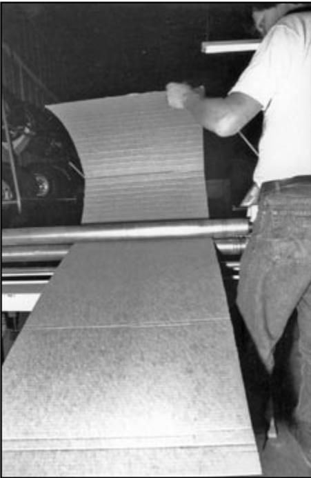
**6** A straight, 24-inch-wide piece of cardboard will simulate each wheel tub's rounded top section. This pass through the Chassiswork metal roller made the cardboard easier to bend into an arc.
