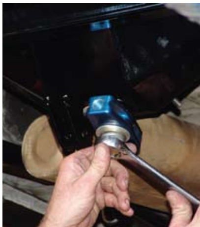
At the forward end of the installation, a bracket that is part of the subframe connector crossmember receives the torque arm.
