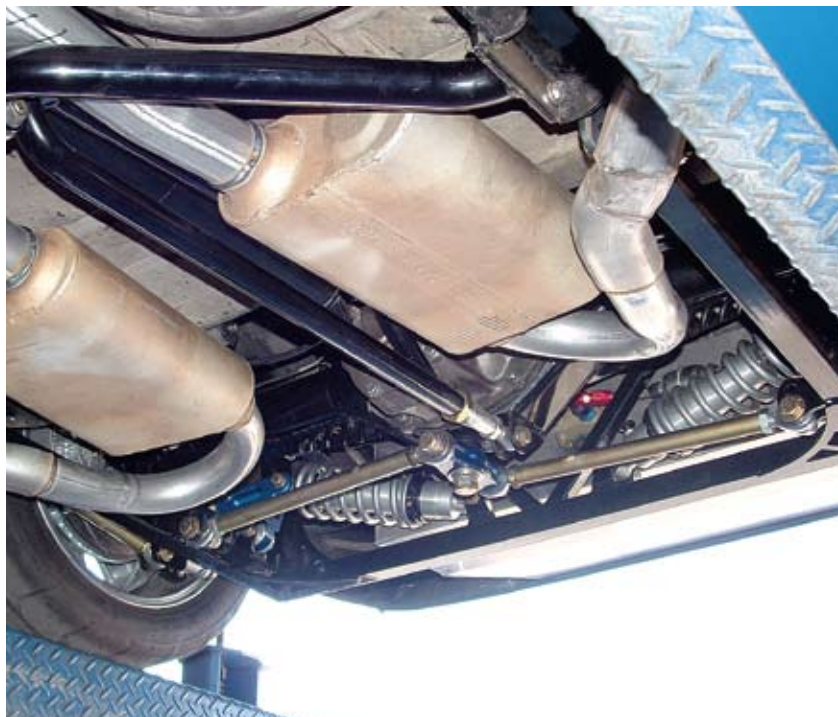
At the forward end of the installation, a bracket that is part of the subframe connector crossmember receives the torque arm.
