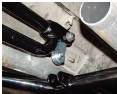
At the forward end of the installation, a bracket that is part of the subframe connector crossmember receives the torque arm.
