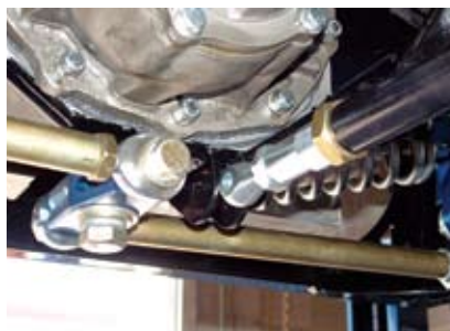
This look at the Watt's linkage mechanism shows the axle torque arm being attached at the axle end.
