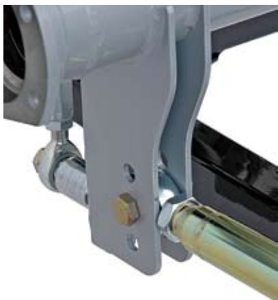
This look at the Watt's linkage mechanism shows the axle torque arm being attached at the axle end.
