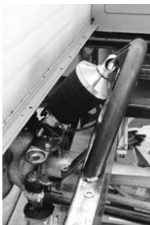
Here's the driver's side and its proximity to the bed side. Here it's deflated and as close as it's going to get. Rodger plans to leave this section of the bed open to show off the polished suspension.
