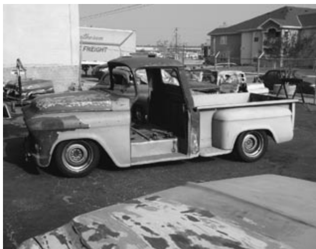
The rake looks good with no air in the bags sitting on 245/50-16 tires. Rodger wants it to lay level when it's parked so that the rear of the frame will get 2'ed when the tubular center section is installed. Stay tuned for part three.
