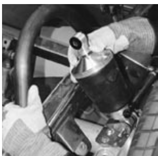
While he was at Victory Circle, Rodger picked up a pair of 1.5-inch diameter U-bends to fabricate the upper mounts. With the suspension bottomed out along with the VariShock, the height of the U-bend was determined, measured, marked, cut and tacked into place. The first hoop was not set at any particular angle, it was "eyeballed" and placed at an angle that looked good. The angle was then measured with a protractor and the opposite side was made to match.
