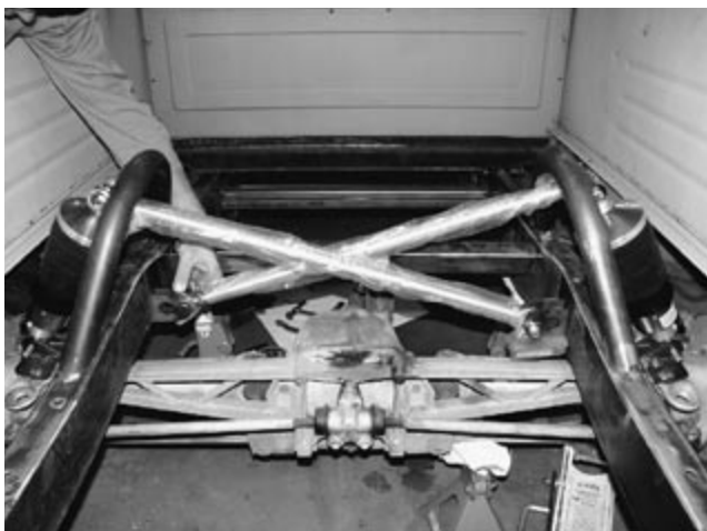
While poking around at Victory Circle, Lee found these sweet aluminum stabilizers and decided to use two instead of one going hoop to hoop. With Heim joints mounted to the ends, they were crisscrossed from each hoop to its opposing framerail using more race shop mounting tabs.
