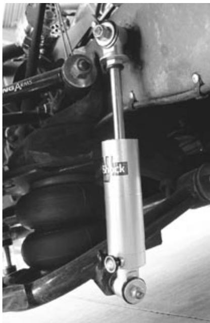
As mentioned, access to the adjustment knobs is easy, especially with the aid of the Air Ride. While we mentioned the settings used for testing, your final combination will probably differ greatly—it all depends on your driving style and ride quality preferences.
