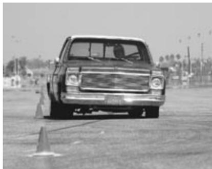
With the VariShocks installed and adjusted (3 clicks compression; 6 rebound), our slalom intervals dropped down to the low 6-second range with an average speed of 43 mph! May not seem like much to you, but in a real-world application, that's a huge difference.
