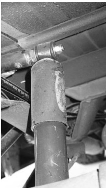
Thanks to the airbags, accessing the rear shocks was made much easier. The new upper mounting studs fab'd by GO-EZ have held up perfectly, which made us feel more comfortable about installing the new shocks on them.
