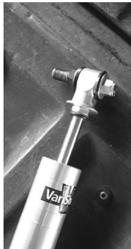
For the front shocks, the C10's stock mounting studs were used, as they have a different size thread on the frame end than the ones supplied.
