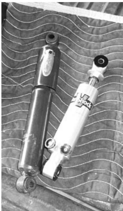
Once our baseline tests were complete, we headed over to a shaded area below California Speedway's huge bleachers for a quick shock-swapping session. With matching bushings, the R&R wouldn't take long. Here you can see the physical difference between the standard tube shocks and the VariShocks.
