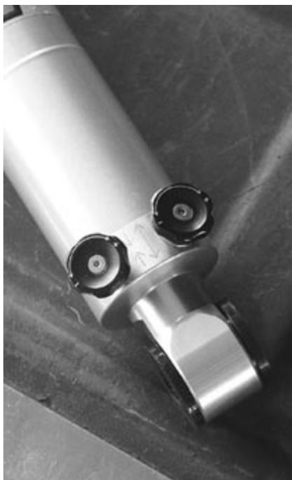
While Alston offers both set and single-adjustable VariShocks, we went with the duals. Because we're dealing with an airbag suspension, we needed independent control of the rebound settings, which neither of the other versions offers. The adjustment knobs are clearly marked and, in our case, easy to access and adjust on the vehicle.
