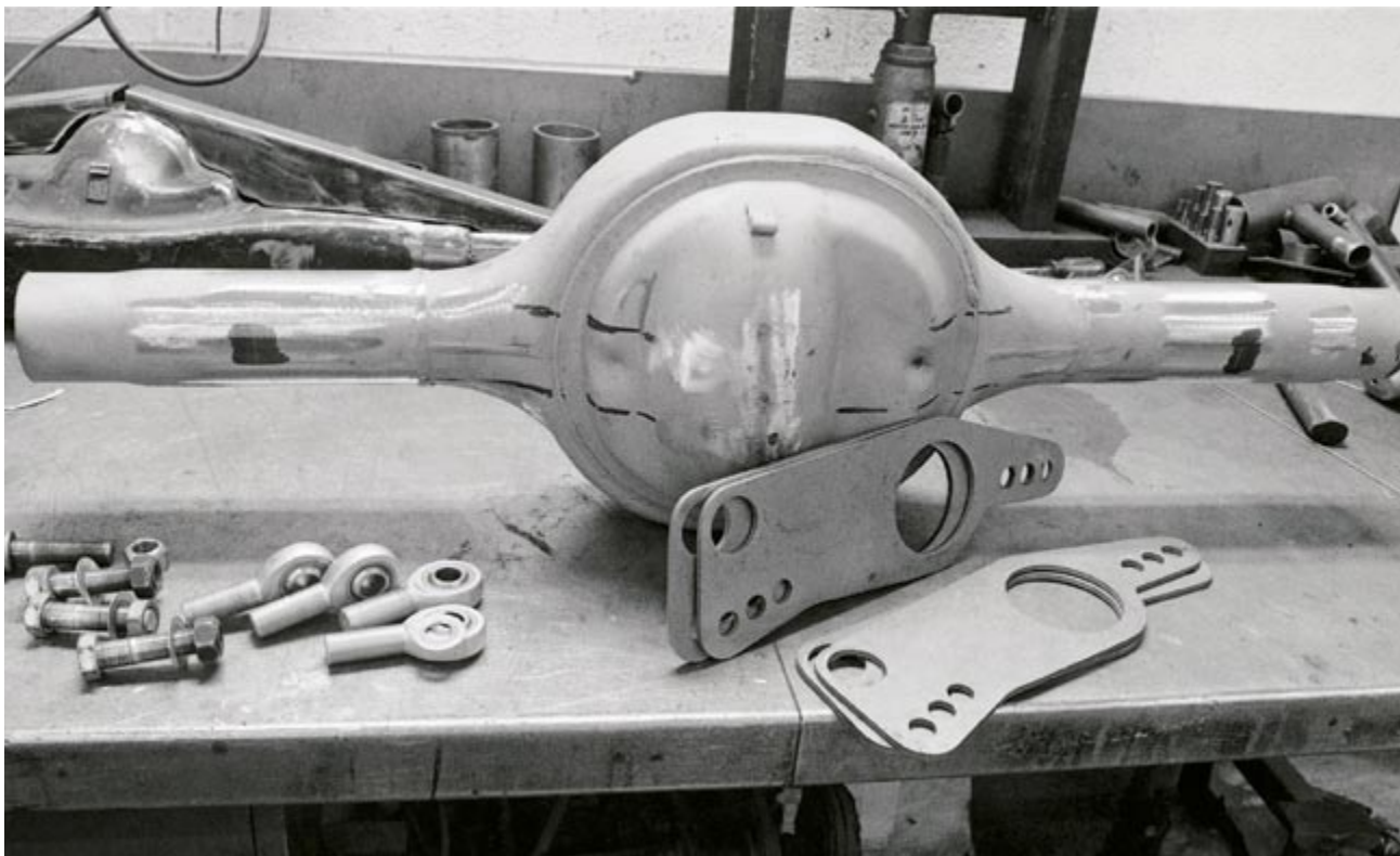
Compare the previous photos of fabricated housings to this shot of a clean junkyard Ford housing. This housing is about to undergo almost a week of surgery before it can be pronounced suitable for a high-horsepower car. Figure the time it takes to repair, then fortify the housing, and you can see just how quickly the fabricated 9-inch housings begin to make sense.
