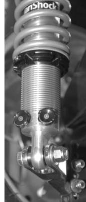
One of the unique feature of the new VariShock is the smaller adjuctment system that not only allows more room around the mounting eyes but also allows greater shock travel within the shock length.
