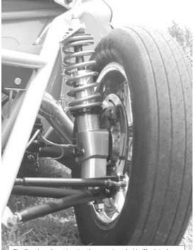
The Chassisworks engineering that went into the VariShock is also incorporated into his new front strut design. The independent bump and rebound adjustment knobs are located at the axle centerline. Note how these racers use a magic marker to note the current settings on the billet strut housing.
