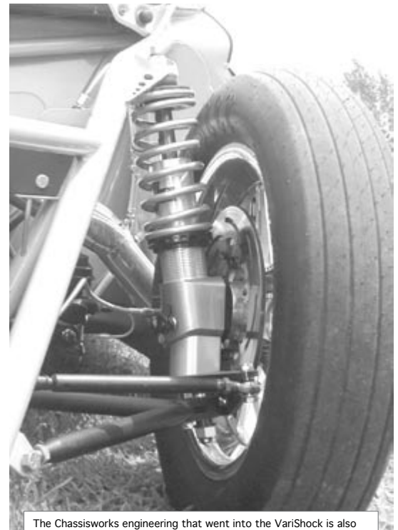
The Chassisworks engineering that went into the VariShock is also incorporated into his new front strut design. The independent bump and rebound adjustment knobs are located at the axle centerline. Note how these racers use a magic marker to note the current settings on the billet strut housing.
