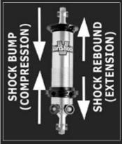
and inhibit weight transfer to the rear tires. By slowly adjusting the bump ratre in on a set of double adjustable front shocks, you can adjuct the rate that the front suspension settles after launch to prevent unloading weight tranfer on the rear tires too quickly.
