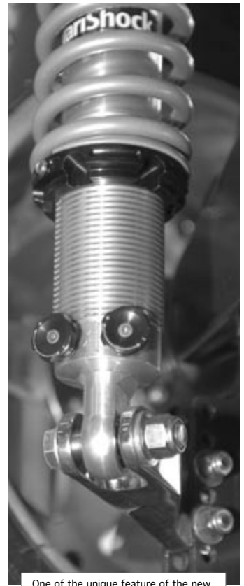
One of the unique feature of the new VariShock is the smaller adjustment system that not only allows more room around the mounting eyes but also allows greater shock travel within the shock length.
