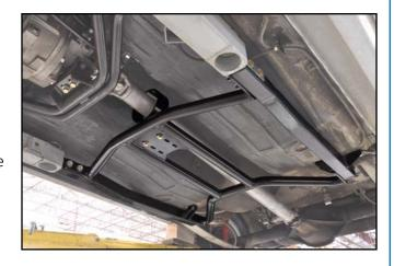
leaf-spring mount sandwiches two of the three gusseted connector mounting tabs against the body, while the third tab attaches using a drilled hole at a stronger, contoured area of the undercarriage. This product ships with a black powder-coat finish, complete with Grade 8 hardware and detailed instructions. Note: This product can be used only with hardtop models equipped with our g-Machine subframe system.
