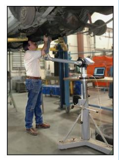
The FaroArm is used to digitally scan multiple vehicles and create an exact computer model for development.
