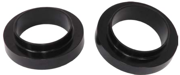
TCP SVM1-03 - 1" thick spring isolators, black urethane, raises ride height approximately 1-1/4"
