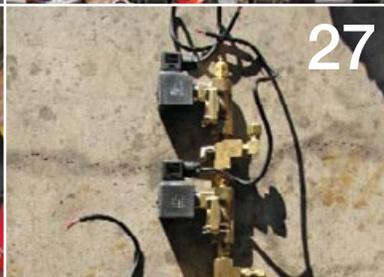
The valves were assembled into a manifold. This means we can have one fill line fill two corners from one assembly. The two completed manifolds (one for front, one for rear) were mounted to the back of the cross member to which the compressors were mounted.
