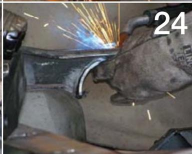
A piece of pipe was cut in half and welded in place to reinforce the cross member.
