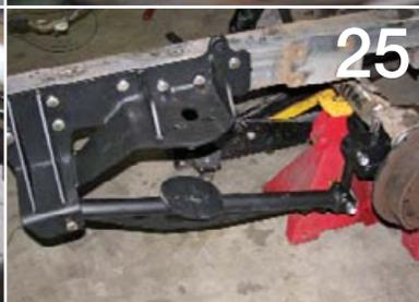
The rear cantilever links were bolted in place. It's important to install the bolts from the inside out so that the bolts won't hit the frame. We also bolted the 'bags in place at this time using the supplied fasteners.
