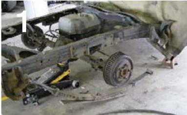
*Next we had to remove the stock shackles. They are held on by rivets, which can either be ground off with a grinder or cut into quarters and knocked out with an air hammer.*
