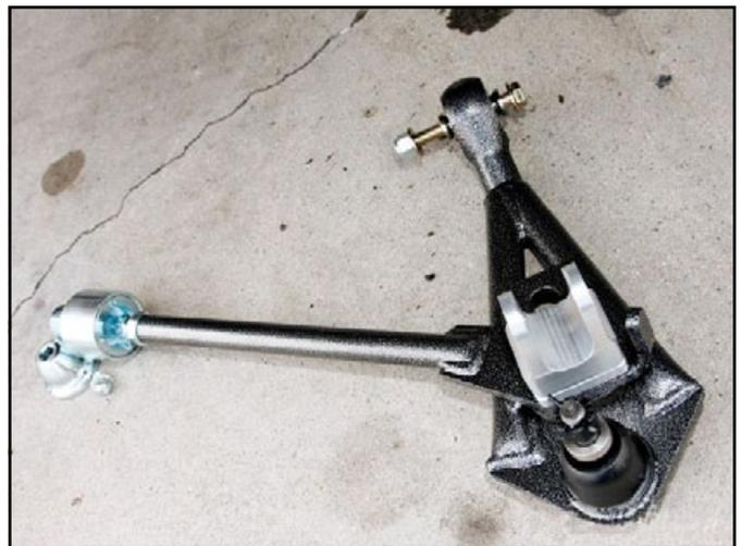
Here is TCP's lower control arm, strut rod, and lower coilover mount assembly. All of these pieces are compatible with factory parts as well as the other aftermarket parts from TCP.
