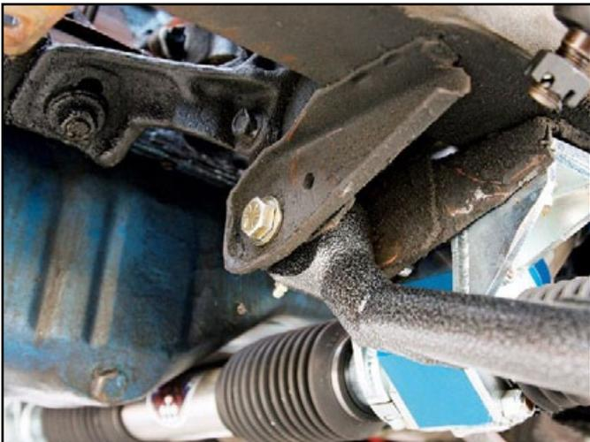
TCP's lower control arm bolts in the same as the factory arm. New bolts come in the kit, but we used the bolts from the rack and pinion system since they are longer than the stock ones. The longer ones are needed to accommodate the rack's brackets.
