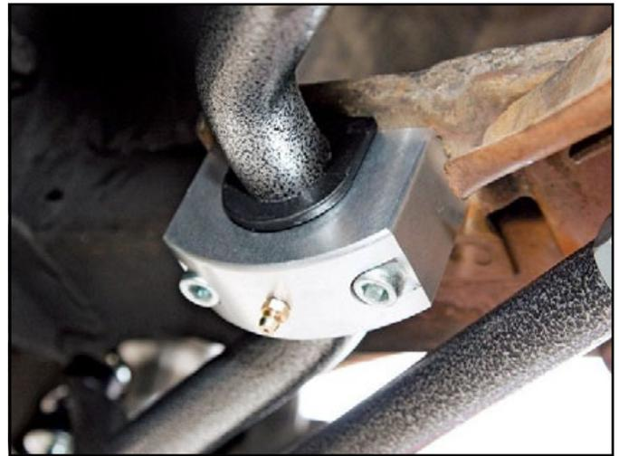
The TCP aluminum frame mount for the sway bar replaces the factory clamp, and uses the same bolt holes. The endlinks go in the exact same way as the factory. This sway bar bolts up very easily, not like in first-gen Camaros.
