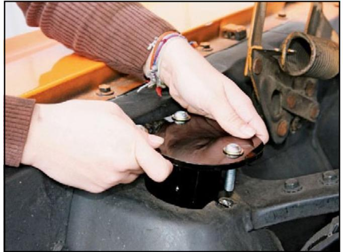
The factory upper shock mount is replaced by TCP's plate that drops in through the top of the shock tower and sandwiches...
