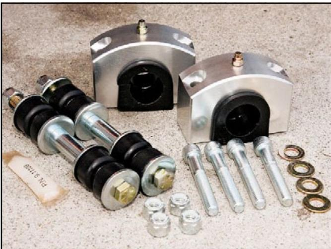
The last part of this project is installing the new sway bar. The kit comes with a 1 1/8-inch diameter bar, billet aluminum frame mounts, endlinks with polyurethane bushings, and all the necessary hardware.
