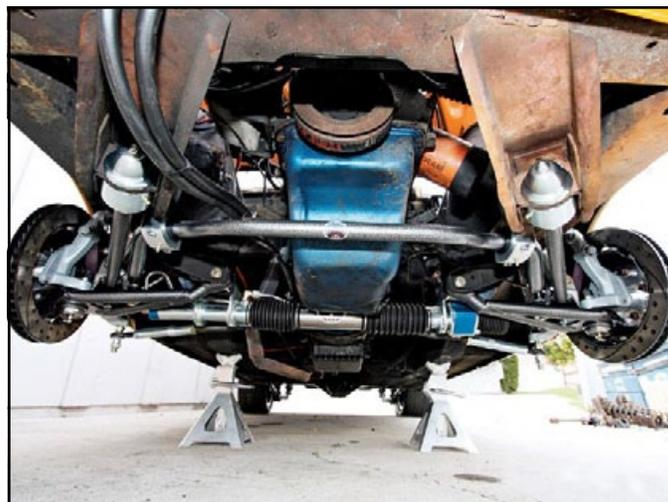
Here's the final TCP coilover front suspension installed in Street Fighter. The new parts from TCP fit perfectly with each other and required zero fabrication. When you've got everything done, go around the front suspension and give each zerk fitting a dose of the good stuff, like Royal Purple's synthetic Ultra Performance Grease.
