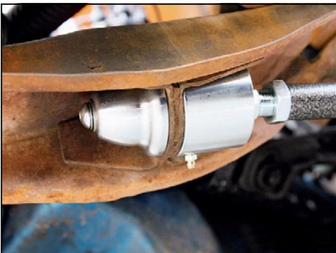
This is the jewel of TCP's adjustable strut rod. It's the first of its kind, housing a Delrin bushing inside the aluminum housing.....
