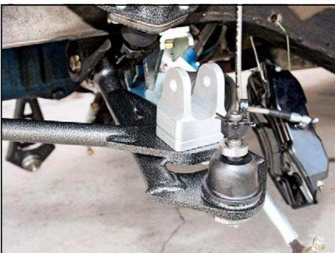
This aluminum bracket is the lower coilover mount. It's threaded to accept the bolts that hold the strut rod to the lower control arm. In a coilover conversion kit without the aftermarket arms, the coilover is mounted between the upper control arm and the body, like the spring is from the factory; that kit retails for \$988.
