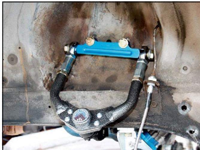
Next in are the upper control arms. You want to adjust the arm to be in the middle of its range. This will ensure everything will fit together; further adjustment will be done at the alignment stage. The arm has a dropped pivot shaft to use the factory pick-up points-this give the TCP system a nice negative camber gain during cornering.
