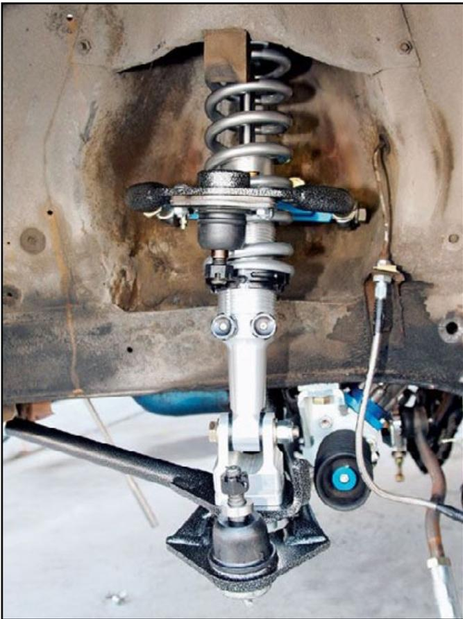
Prior to this photo, we ran the suspension through its travel without the spring installed to check for any binding. You need to make an educated guess of how much space the spring takes up while doing this test. If everything looks good, install the spring into the coilover, then into the car.
