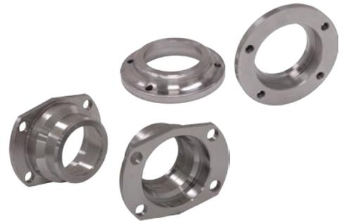
▲ These are some of the housing ends manufactured in-house at Chassisworks and available off the shelf. The sealed-style ends (upper group) allow the use of the stock axle seals and wheel bearings. Drag-style ends (lower pair) are intended for use with sealed bearings to allow narrower housing widths.
