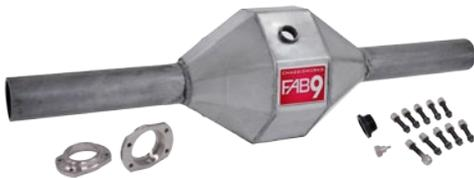
▲ This is an "unassembled" FAB9™ as it is delivered to the customer. The short-tube, mild-steel housing is fully welded and comes complete with all necessary hardware, including the threaded drain and filler plugs, and a pair of housing ends appropriate for each particular application.
