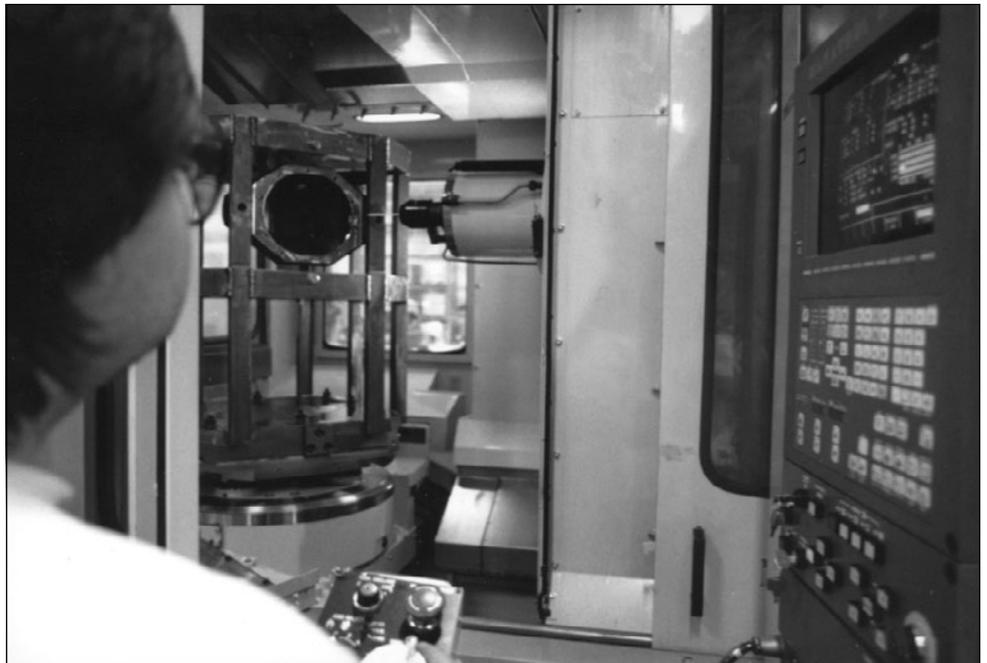
▲ The FAB9™ housing is automatically loaded into the machine's huge working area. After being rotated into position, this ruby-tipped sensor verifies its location before the work commences.
