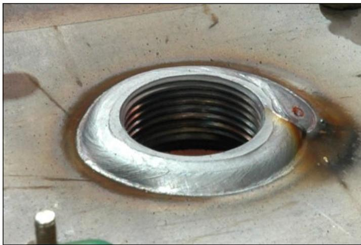
▲ This close-up of the center-section filler port clearly shows the quality and accuracy of the welding found throughout the FAB9 center section.
