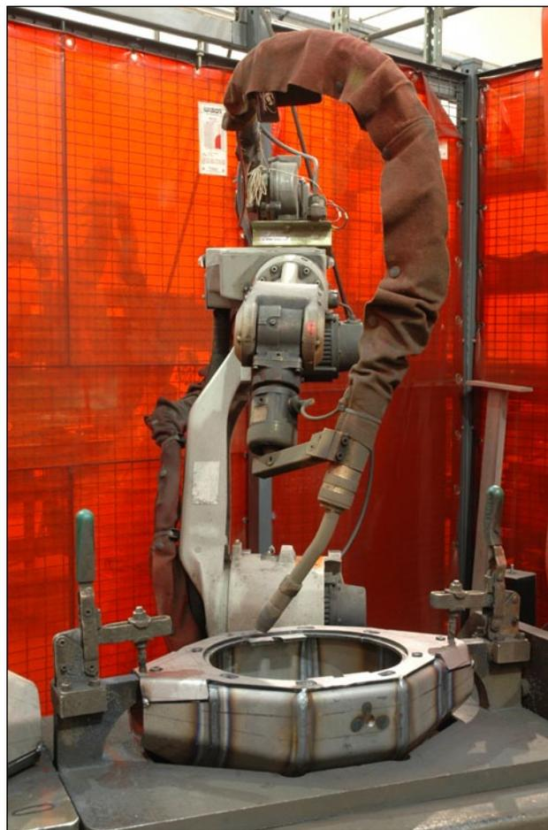
▲ To best control the quality and consistency of the welds on an assembly with extremely high performance demands such as the rear end center section of a drag-race car, Chassisworks puts to use an array of robotic spray-arc welders with auto-rotating fixture tables. This marvel of manufacturing technology creates perfect welds every time and significantly reduces the amount of man-hours that factors into the cost of the final product.
