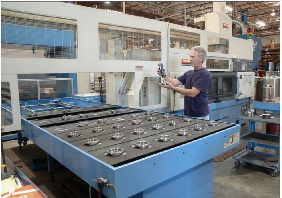
▲ This is one of the supertrick, robot-fed CNC machines that are used to turn billet-steel "hockey pucks" into ready-to-use housing ends. Amazingly, it takes just about as long for the automatic saws to cut each blank as it does for this Mazak Multiplex to transform it into a finished part.
