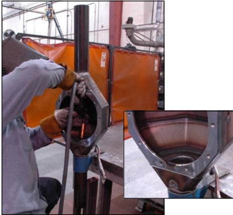
▲ Welding the axle tubes to the inner bulkhead, (arrow) as well as to the end of the housing, results in unprecedented strength, as does the FAB9™'s beefy, fully supported gearset-mounting flange.
