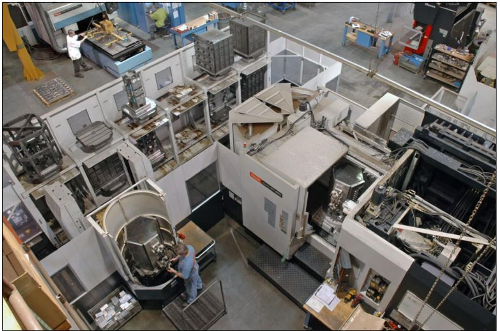
▲ After the housings are welded up, they make a pass through this giant Mazak Palletech manufacturing cell for the final machining steps. Weighing well in excess of 30 tons, which doesn't even include the robot-loading conveyer components, this monster required its own rubber-isolated, two-foot-thick, 12-foot by 24-foot concrete foundation. Along with occupying a fair amount of the Chassisworks facility, it also pretty much dwarfs its operator.
