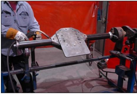
▲ Once a pallet is full of machined housings, a forklift brings them into the welding area. The use of this rotating fixture helps in achieving perfect alignment and sanitary welds.
