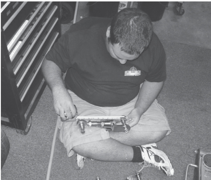
^ Both the ProPower uppers and lowers are double-adjustable, meaning that they can be lengthened or shortened while still on the car by backing off the jam nuts and turning the center section, turnbuckle-style. To make sure we had the full range of adjustment available after they were installed, we made sure we had the same number of threads showing on each end, then turned the center section until we had the right center-to-center length: 9-13/32 inches for the uppers, and 17-11/16 inches for the lowers.
