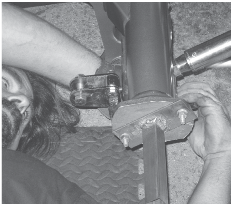
^ The other ends of the arms connect to the Fab9 housing just like you'd expect - up top, spherical bearings connect the UCA's (you can also order a Fab9 set up for conventional-style bushings) and the LCA's bolt into stock-style mounting pockets on the underside. One nice feature of the Fab9 is that there are two different mounting positions for the lowers to allow a modicum of adjustment of the instant center.
