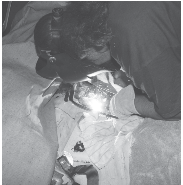
^ With the plates bolted securely in place, we stitch-welded them around the perimeter, then painted the new steel and exposed floorpan to keep them from rusting. Now, we were finally ready to hang the new rearend and suspension.
