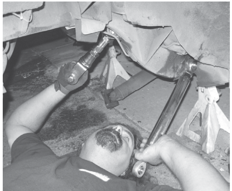
^ The control arms go in just like the stockers, but rather than being located by soft bushings, spacers and spherical bearings carry the load. You'll note that the lowers are equipped with offset spacers that move the arms toward the centerline of the car, which provides additional clearance for big tires. Chassisworks offers separate lower control arms for older-style 12mm chassis mount bolts, or the newer 14mm style, so be sure to check which ones are correct for your application.
