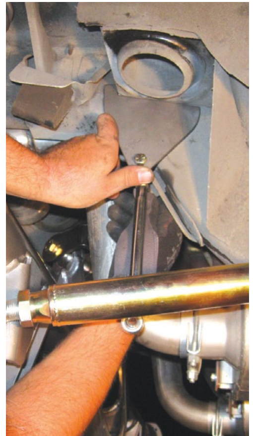
^ The anti-roll bar end links mount to the chassis via sheetmetal plates, which must be welded to the frame rails alongside the stock upper spring perches. The links themselves are double-adjustable, and connect to the solid 1.25-inch steel bar via 8.2-inch long (center to center) billet aluminum arms.
