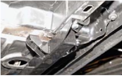
With sub frame connectors fitted in place, the mounting holes are drilled, and the combination 3/8-inch and 7-20 x 3-inch bolts are bolted into place.
