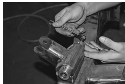
Next, Maxwell repeats the thread chasing process on the control arm mounts because any time in manufacturing, a small burr can get inside, and potentially damage potentially expensive fastener hardware. Just call it a safety precaution, folks!
