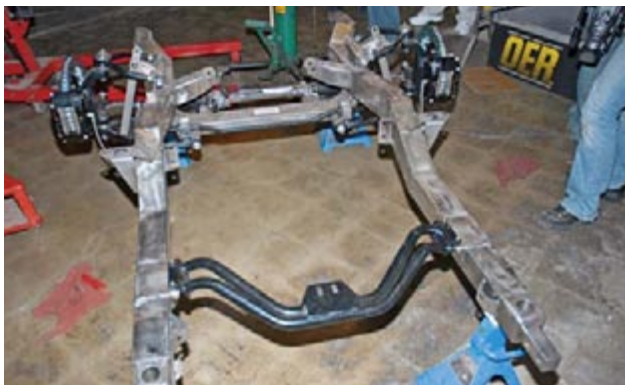
Prior to dropping our 502 big-block power train into place, Woods and Maxwell install the Chassisworks transmission cross member using the provided bolts in the Chassisworks kit.
