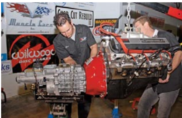
Now it's time to join together the 'Gem's GM Performance Parts 502/502 big-block and Keisler TKO 600 tranny.
