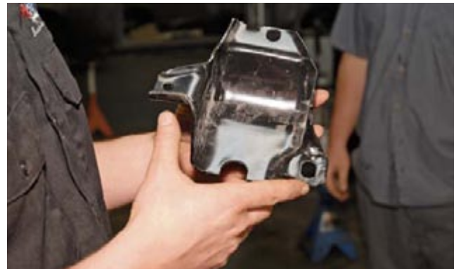
On the opposite end our crew installs the OE reproduction spring bucket for the Camaro rear leaf springs to "sit" in using the OE bolts provided.
