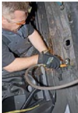
In the process, some seat clearance issues were addressed with the floor pan. A couple of slots were cut prior to bolting up the sub frame connectors.
