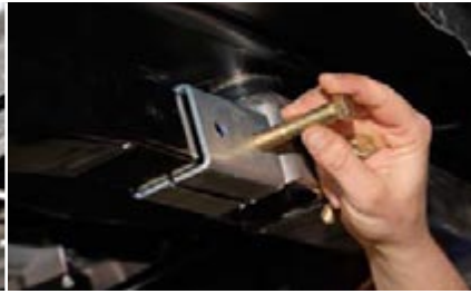
With sub frame connectors fitted in place, the mounting holes are drilled, and the combination 3/8-inch and 7-20 x 3-inch bolts are bolted into place.
