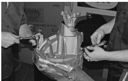
With the carrier in place, it gets snugged in place via a series of 3/8-inch Nylok nuts.
