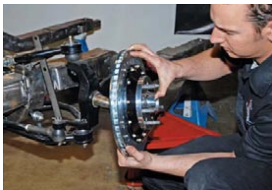
Bret installs a completed rotor onto the correct spindle keeping in mind that they are directional. To fully set the bearings, the accompanying castle nut should be final torqued to 12 lb/ft while spinning the rotor in the forward direction. This will remove any excess grease that could cause wheel bearing play. The castle nut is then backed off to the "just loose" position which should produce the desired .001 to .005-inches of end play. Finally, the cotter pins are installed.
