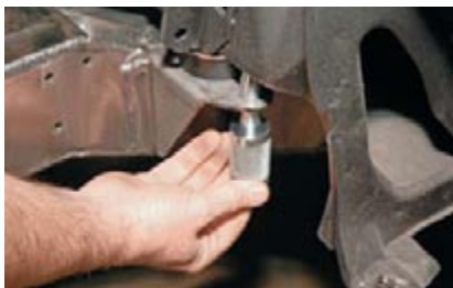
Another of the pleasing features about the Chassisworks F-Body sub frame is that the manufacturer provides the builder with a pair of 5/8-inch threaded frame alignment pins, invaluable items for all important pre-assembly.
