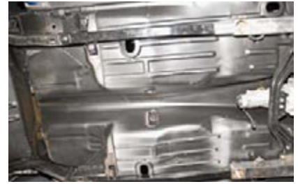
With sub frame connectors properly bolted up, they should butt up to the Chassisworks front sub frame like this.
