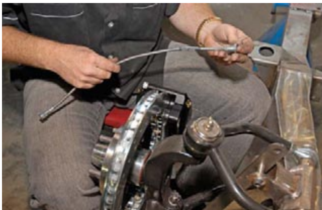
With that done, we see the installation of the provided 3/8-inch, braided stainless brake lines.
