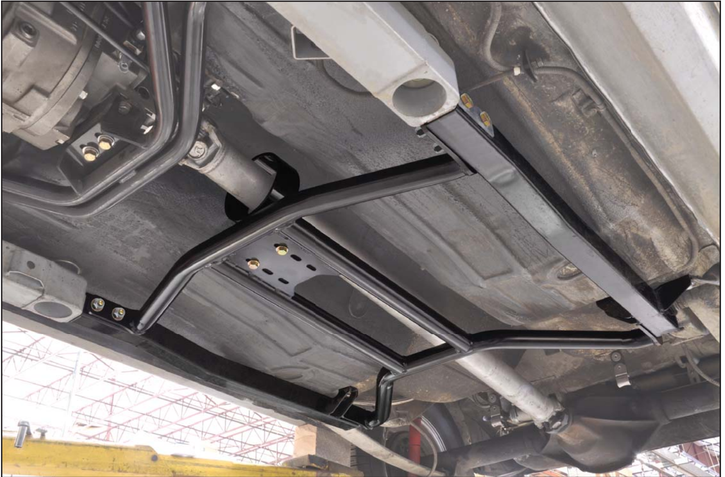
Image shows non-torque arm center support.
