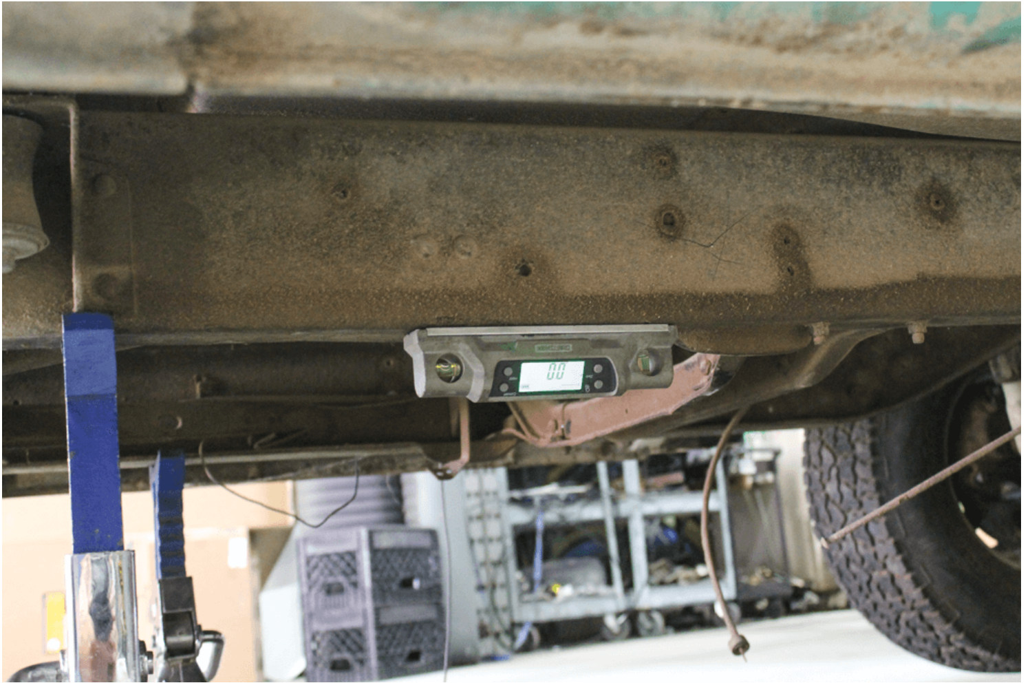
04 We placed the stock chassis on jack stands and leveled it in both directions: left to right and front to back.
