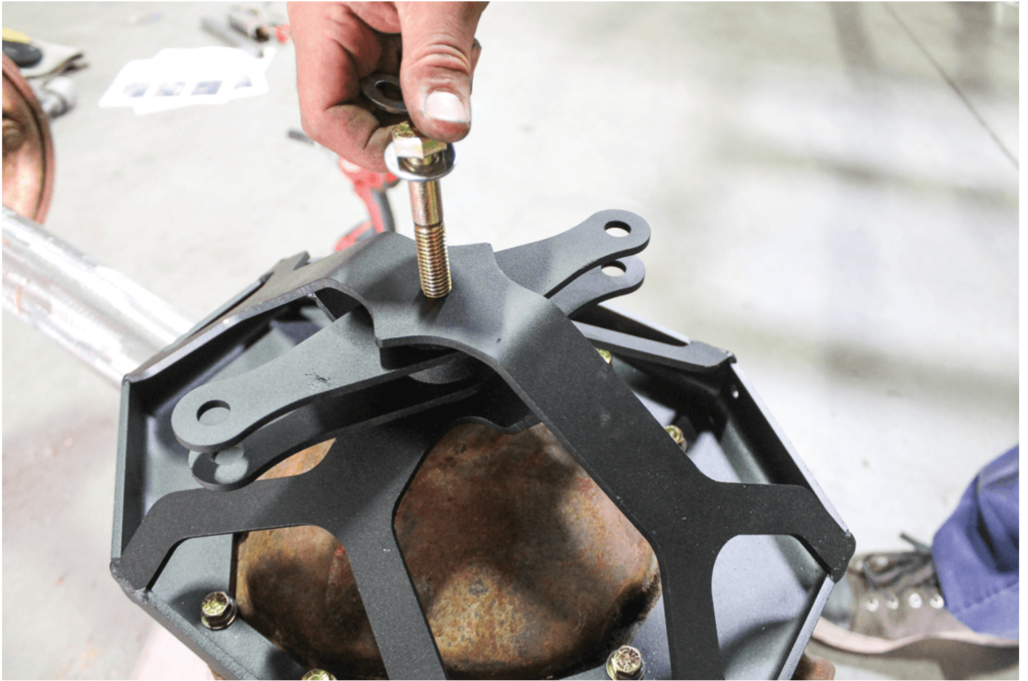
The actual pivot was slid in between the mounting surfaces and bolted in with the new hardware.
