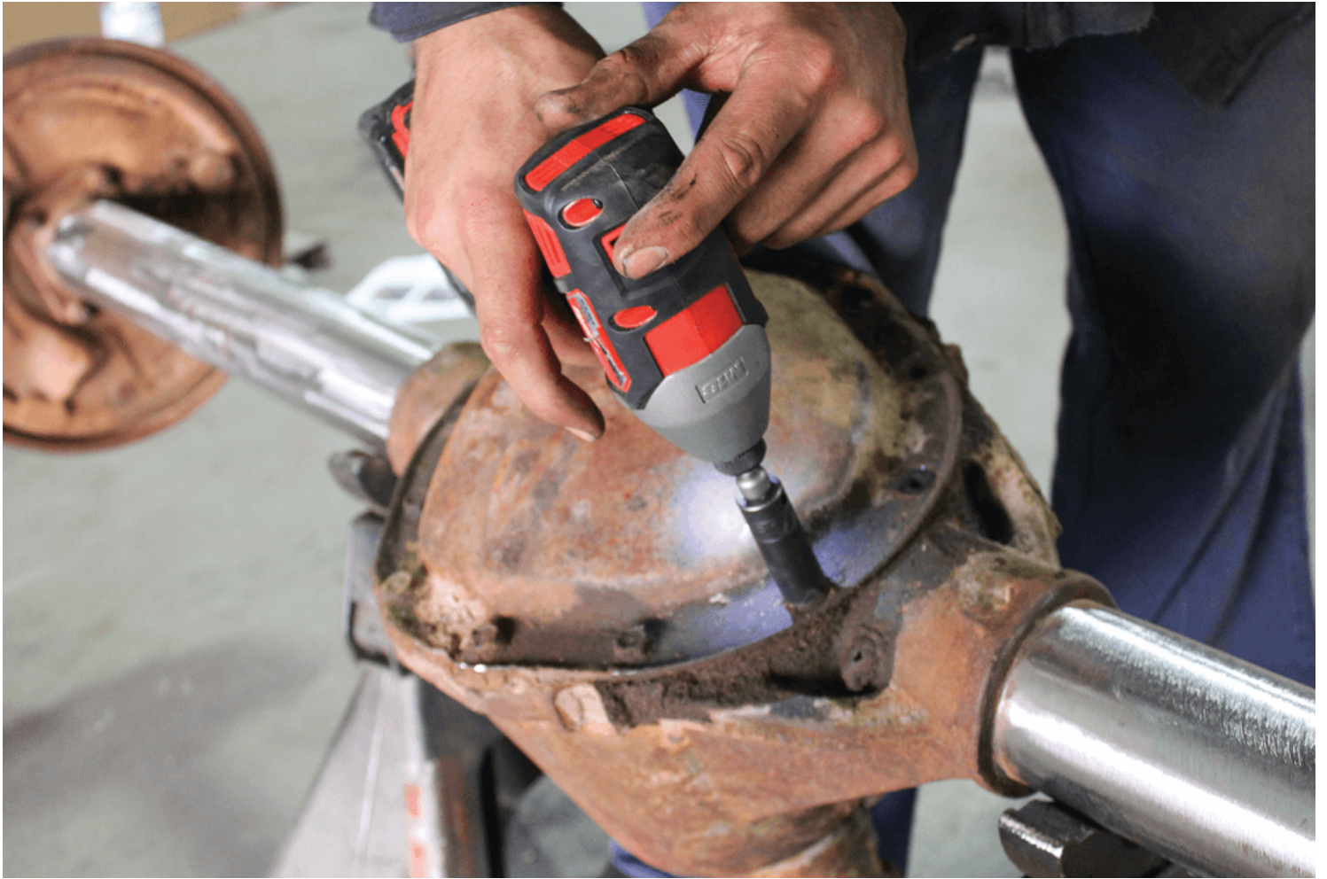
Installing the brace for the center pivot of the Watts-link required the removal of the differential cover hardware.
