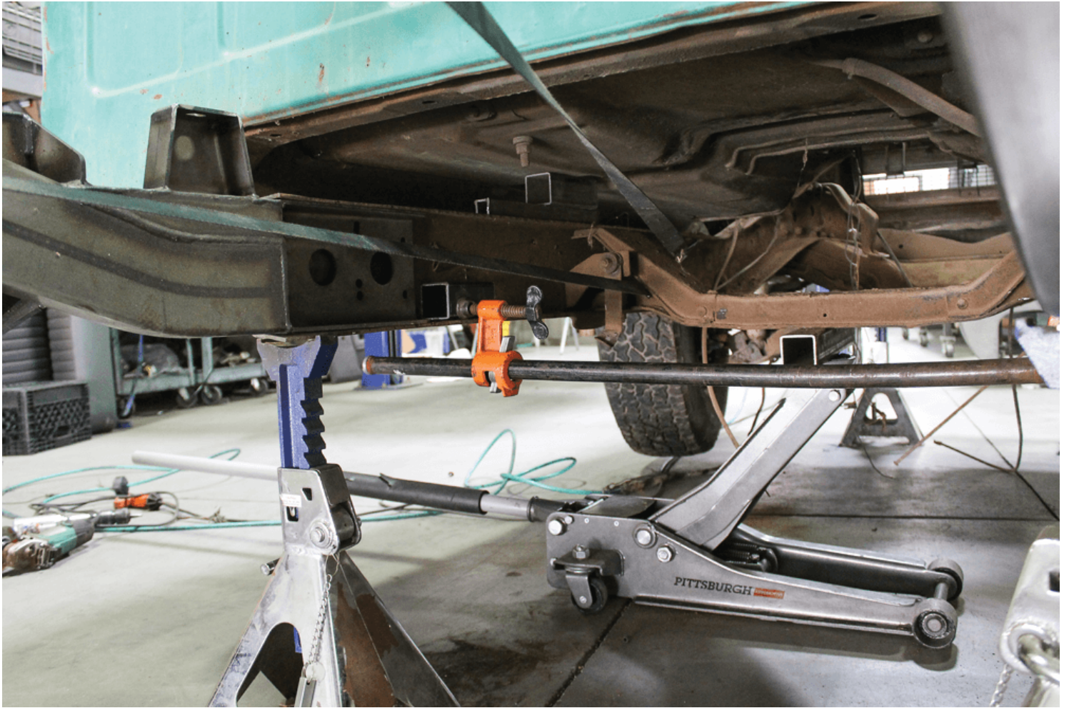
Using spreader clamps, we got creative and spaced the frame just enough to slide it in the rest of the way.
