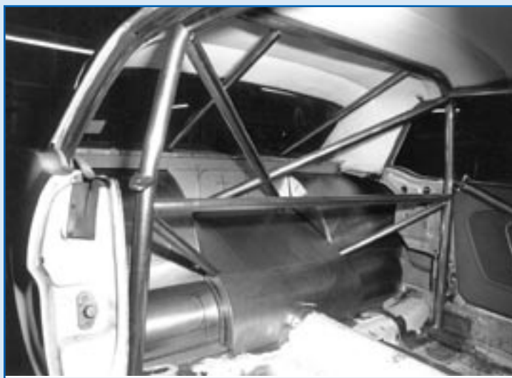
Cleco clips hold the various panels in place, pending powder coating. The rear firewall was custom-built. (Chassisworks has since added a production firewall to its interior kit for this application.)
