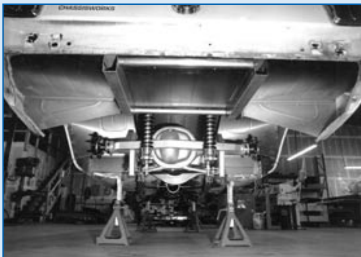
Following powder coating, the wheel tubs, belly pans and floor sections will be riveted to the frame and sealed with silicone.
