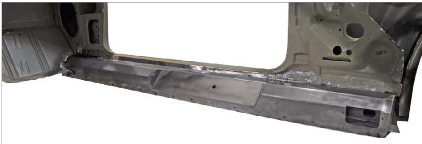
Firewall Rocker End (left): The new rocker extends through the firewall and features a large support gusset.
