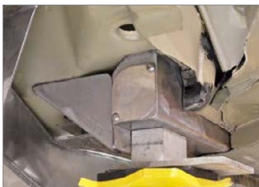
Firewall Rocker End (left): The new rocker extends through the firewall and features a large support gusset.
