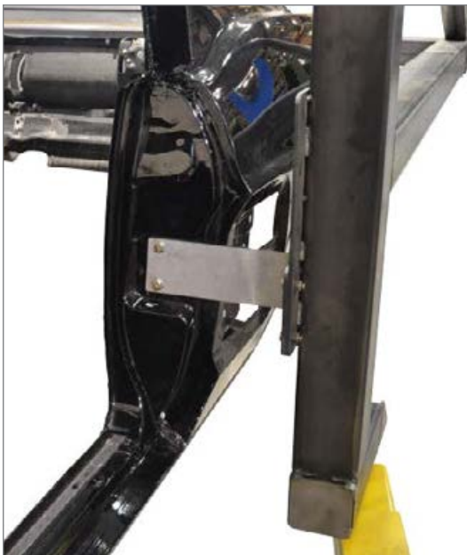
B-pillar (door striker) body adapter
