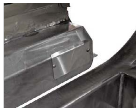
Stainless Caps (left/right): Access holes at each end of the rocker allow wiring or plumbing to be safely routed through each rocker structure. Removable stainless steel caps are provided for easier installation of bulkheads or grommets.
