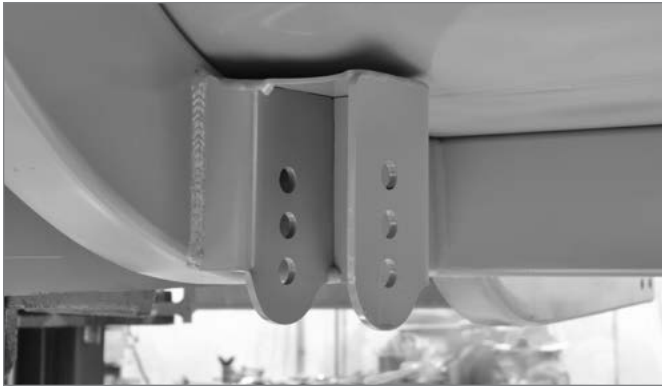
3-Position Lower Control Arm Mount
