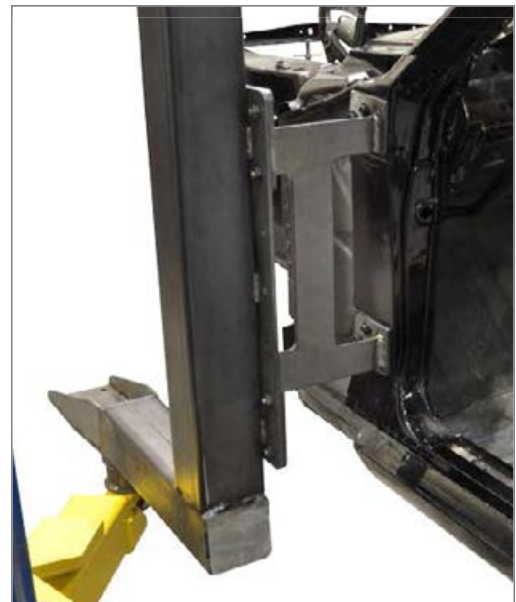
A-pillar (hinge bosses) body adapter
