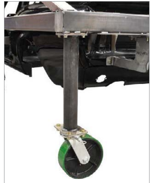
Rear caster with extended fixture legs
