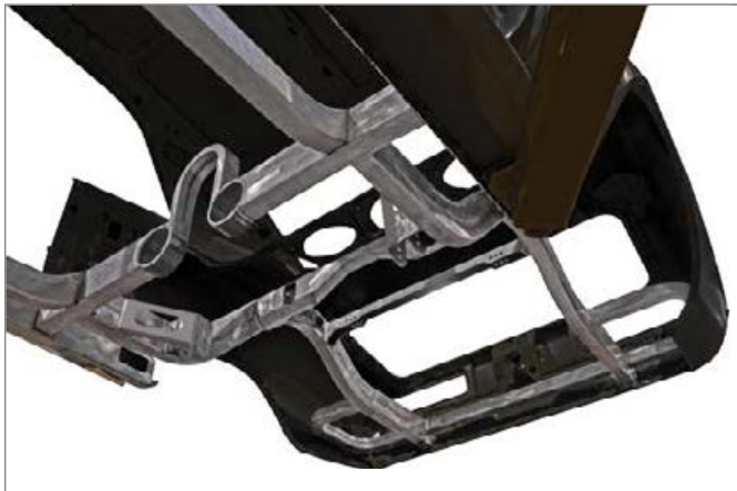
Tall driveshaft loop allows body to sit lower over the drivetrain without risk of driveshaft contact. Crossmember features factory-welded, dual 4"-ID exhaust ports.
