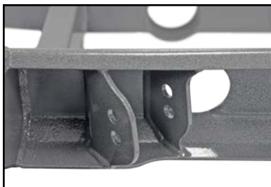
Two-position upper-link mount enables simple adjustment of suspension instant center.
