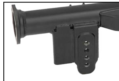
Four-position shock mount plate with reversible clevis (not shown) for eight different settings.
