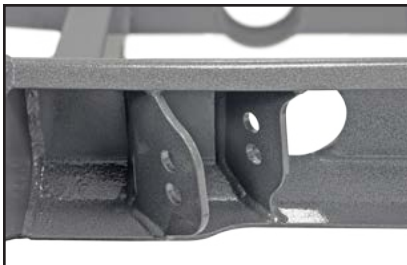
Two-position upper-link mount enables simple adjustment of suspension instant center.
