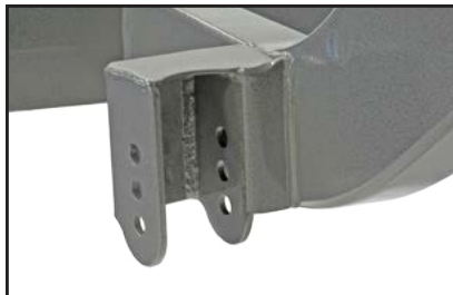
Three-position lower-link mount used with three-position housing mount for nine different settings.
