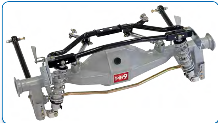
Coil-Over g-Link with FAB9 Housing
