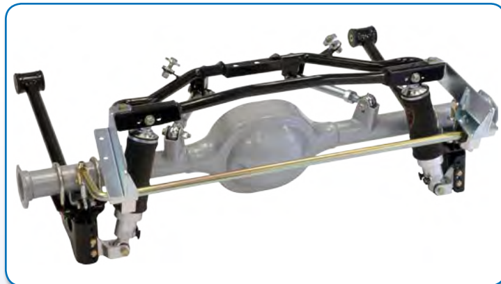
Air-Spring g-Bar with OEM Housing
