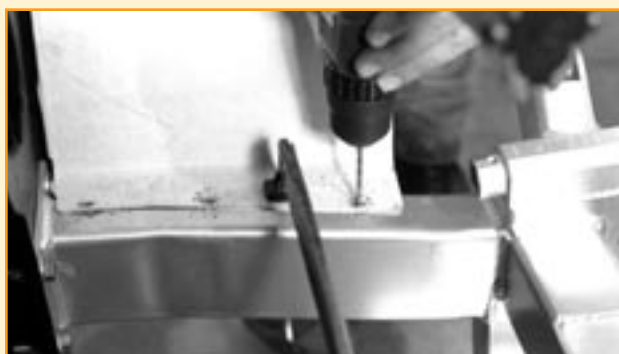
No welding, but some drilling required. The holes drilled into the frame, through the slots in the inner splash panels, are then tapped for the 10-32 stainless screws that are provided.
