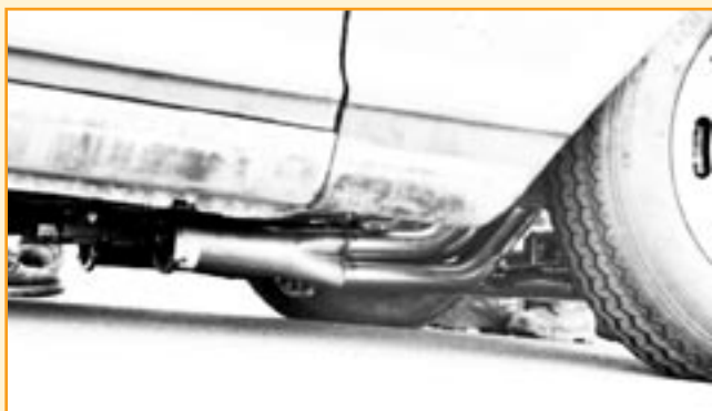
With this Nova back on the ground and rolled outside, the ground clearance under the headers is evident.
