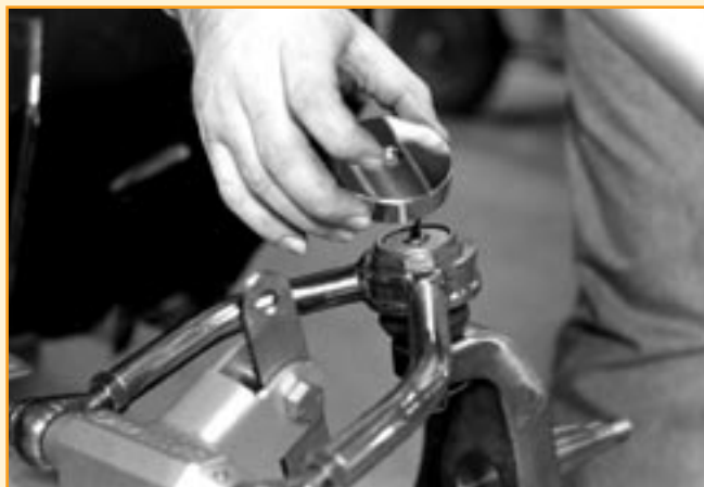
After greasing the balljoints, the zerk fittings are removed. These stainless-steel caps are secured with countersunk stainless screws.
