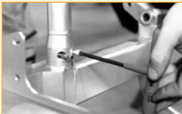
Special high-strength-steel, socket-head Allen bolts are used to secure the struts solidly to the frame.
