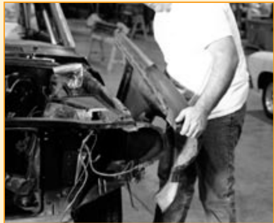
Once the car's steering column, hood, grille, bumper and headlight assemblies are removed, the fenders are the next to go.
