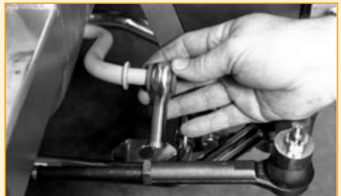
We manufacture the antiroll-bar-link eyebolts in-house. Urethane bushings are again used, and the eyebolt mounts to the pad visible on the lower A-arm. Also visible is the tie-rod end.
