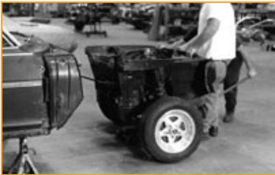
This is the assembled look of our true-bolt-on front frame for the 1962-67 Chevy II. Absolutely no welding is required to achieve professional-quality results with this kit, which also removes around 50 pounds from the nose.
