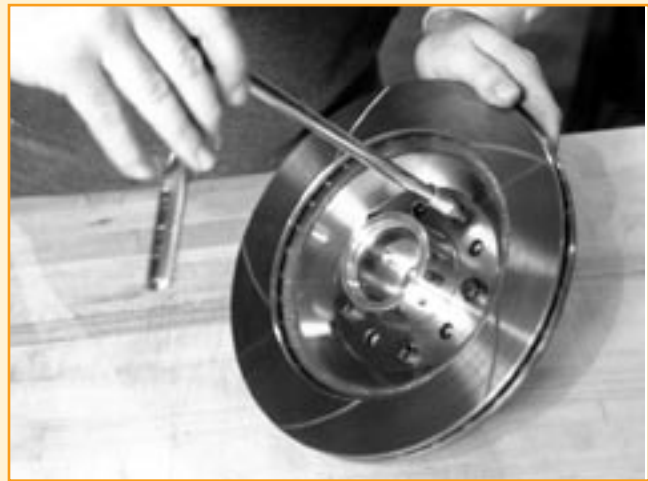
Our 11-3/4-inch, vented rotors are directional, and drilled for both bolt circles.
