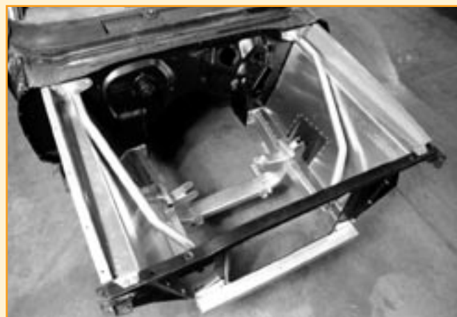
It's amazing what can be achieved these days without a welder. The abundant space in the engine bay is also readily apparent.
