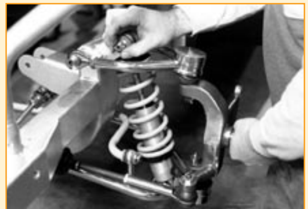
After checking the suspension, adjustable coil-over shocks are installed.
