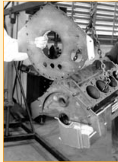
Shown here is a Bolt in midplate for the Lakewood bellhousing, also available is a midplate for automatic transmissions.
