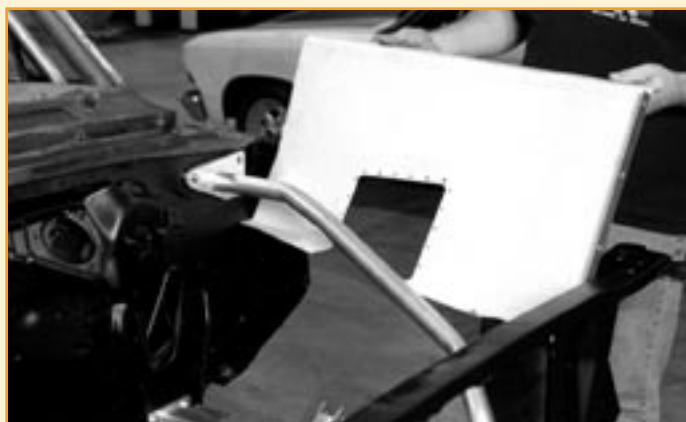
Our preformed and predrilled aluminum inner splash panels slide down into place...
