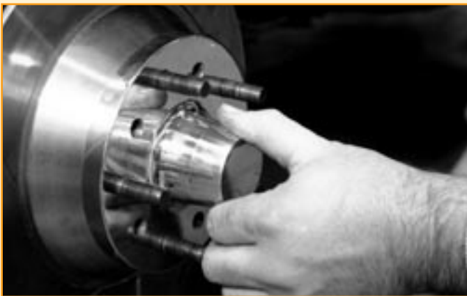
After greasing and installing the wheel bearings and mounting the hub/rotor assembly on the spindle, a dust cap is screwed hand-tight onto the hub; an internal O-ring will keep it from coming loose.
