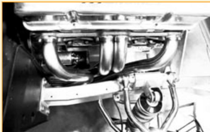
...while the passenger side clears the aftermarket mini-starter.
