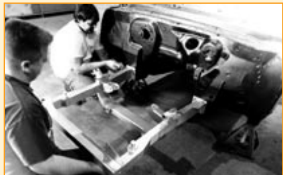
After treating the firewall to a cleanup and fresh coat of paint, the new, factory-welded main-frame segment (which includes all the suspension mounts) is simply held in place as it is bolted to the car.
